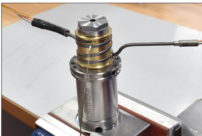
Picture 105: Coated tip of thermocouple
