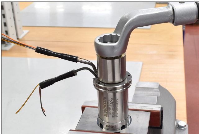
Picture 108: Clamp the nozzle, disassemble the adapter
