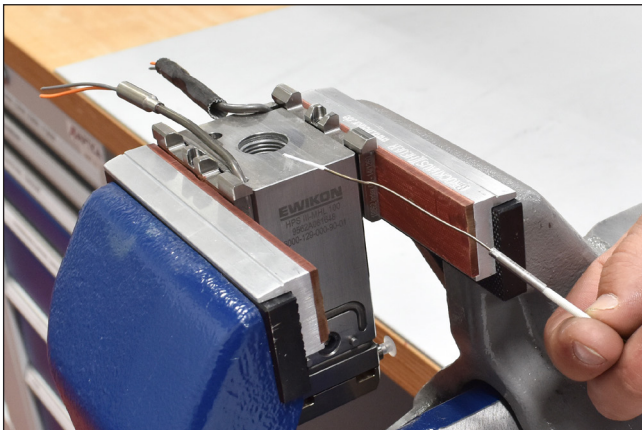
Picture 98: Coated tip of thermocouple
