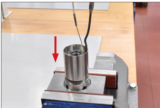
Picture 112: Installation of the new thermocouple, installation of the protective tube
