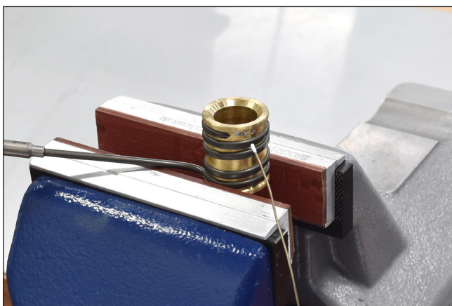
Picture 93: Coated tip of thermocouple
