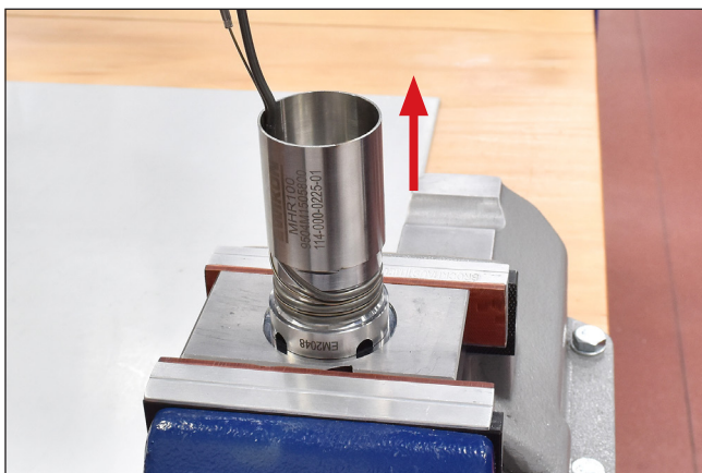
Picture 110: Disassemble the protective tube
