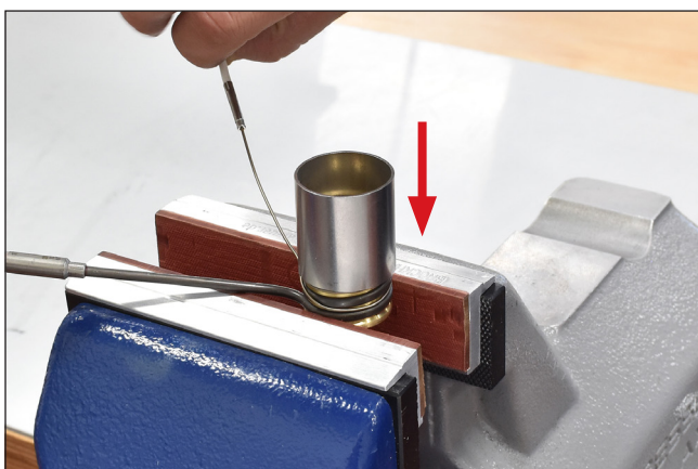
Picture 95: Installation of the protective tube
