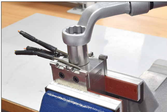
Picture 88: Clamp the nozzle and unscrew the adapter
